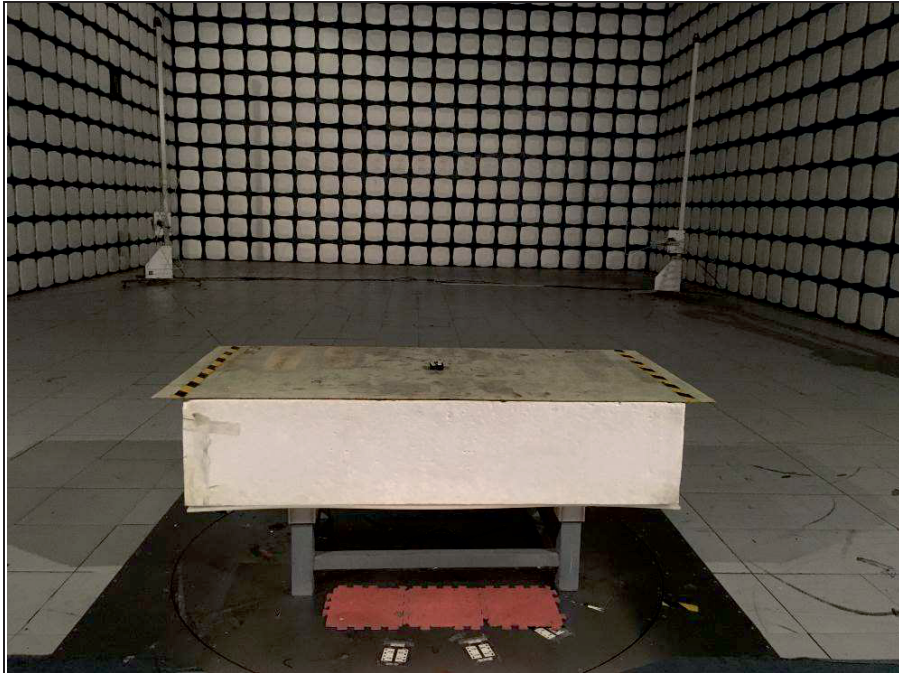
RADIATED EMISSION TEST < 30MHz~1GHz>
